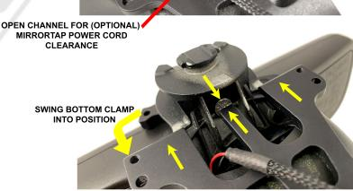
2 - We recommend sitting in the passenger seat when installing this mount and placing a towel over the dashboard. If you are installing a MirrorTap Power Cord to power your radar detector, it needs to be installed before installing this mount. Remove the bolt from the right side of the bottom
